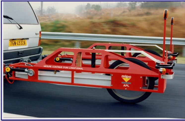
Measured by Longitudinal Profile Analyser (APL*)
