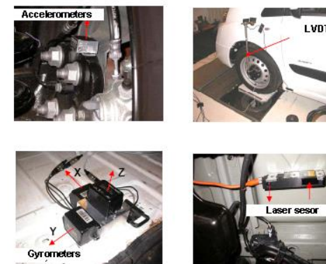
The installed sensors
