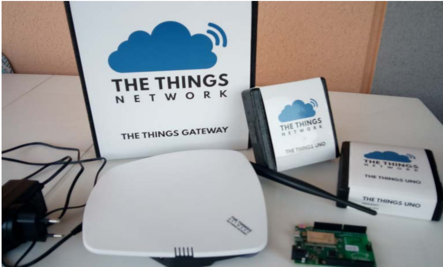
LoRa Gateway and Nodes used to deploy our network
