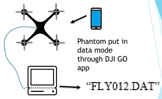
Connected to forensic workstation using USB cable, forensic image created using DD tool (very slow!)
