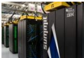
Summit - IBM Power System AC922, IBM POWER9 22C 3.07GHz, NVIDIA Volta GV100, Dual-rail Mellanox EDR Infiniband
