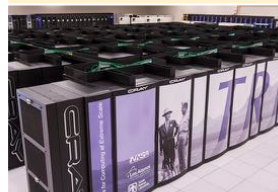
Trinity - Cray XC40, Xeon E5-2698v3 16C 2.3GHz, Intel Xeon Phi 7250 68C 1.4GHz, Aries interconnect h
