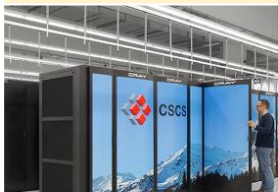
Piz Daint - Cray XC50, Xeon E5-2690v3 12C 2.6GHz, Aries interconnect, NVIDIA Tesla P100
