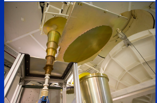
Fig. 2-12. Goldstone 70-m antenna XTR cone X-band HEMT amplifier.
