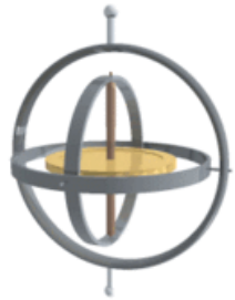
Gyroscope: Sensing angular velocity
