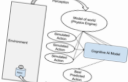
Figure 3. Diagram of PACT-R concept, environment is simulated and simulated actions are used under the control of a cognitive model.
