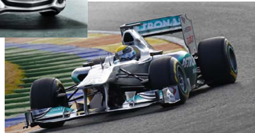
2009 Mercedes-Benz Formula 1 with KERS hybrid energy recuperation system.
